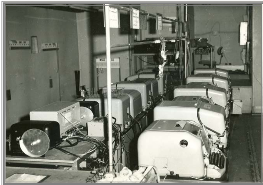
C-11B, Communications Center fabricated from a C-119 Aircraft Simulator
