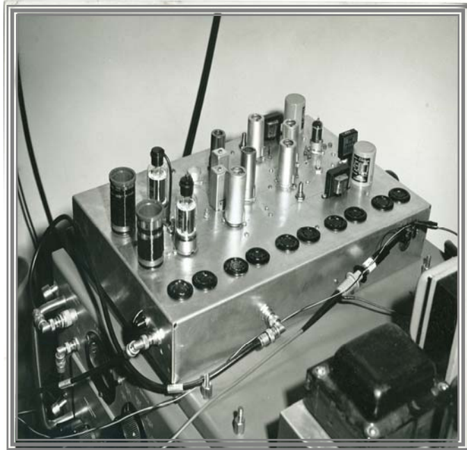
274 th CS Modification of a Collins Radio AM Transmitter T-368 to Single Sideband
